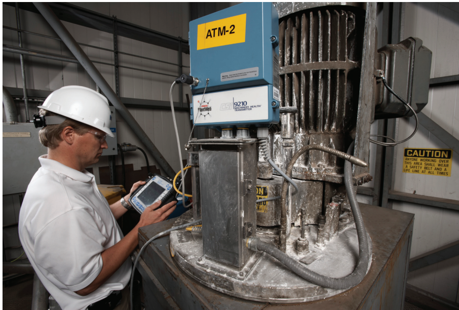
Figure 4 - Checking Vibration Readings at Atomizer 2.
