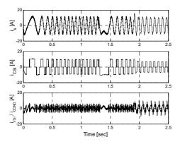
Fig. 6. Current waveforms in a motor phase and at the output of the CSI and VSI/condensers.
