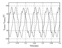
Fig. 16. Condenser-voltage d-q components time diagram after reconfiguration.
