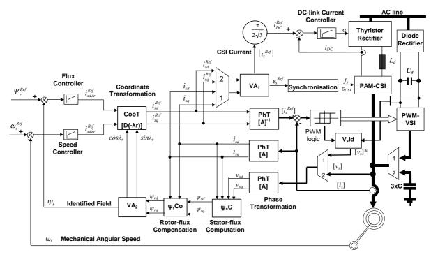
Fig. 1. Reconfigurable vector control structure with two configuration states.
