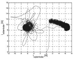
Fig. 5. Stator-current space-phasor diagram in the rotor-field-oriented reference frame.
