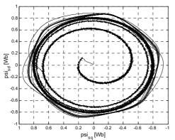
Fig. 11. Stator-flux space-phasor diagram in the stator-fixed reference frame.
