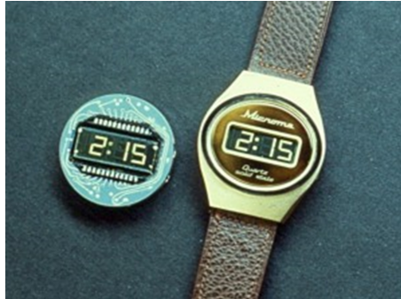
Figure 1.3: The first wristwatch equipped with a dedicated SoC: The Seiko Microma in 1974 [Pre14]
