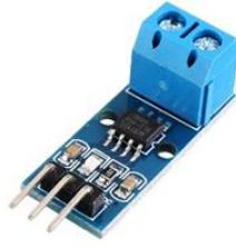
Figure A.6: ARD-000635 Current sensor unit.
