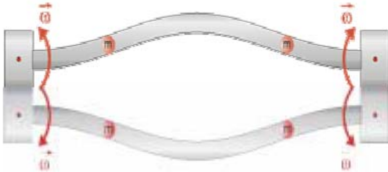
Figure 1: Dual tube design with zero flow
